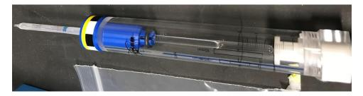
2. Put the NMR tube into the Samplecase holder and remember the holder number
